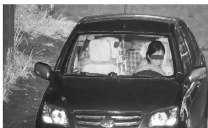
Penetration through window film at night
