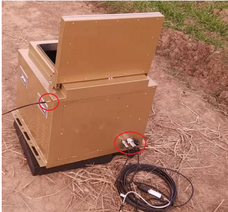
Figure 4 Integrated Storage-Transport-Launch Container and Interfaces
