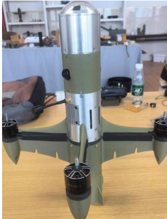
Figure 3 External View of Electrically Propelled Drone
