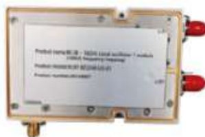
0.38-18GHz/Ku/Ka band local oscillator module (frequency hopping)
