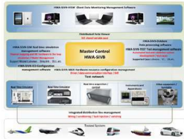
HWA-SIVB Integrated Verification Platform of Simulation Test System
