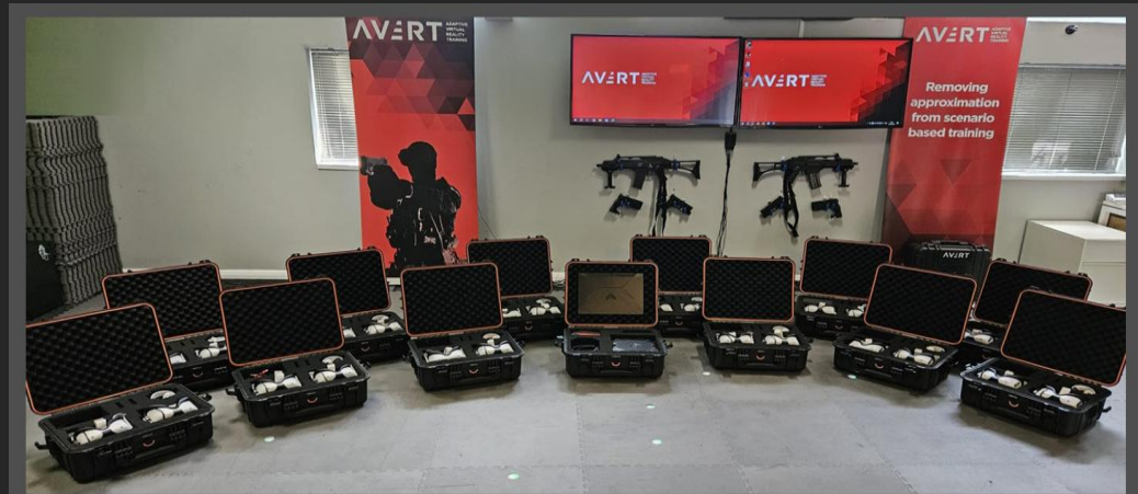
The AVRT Command Pack and all 12 AVRT HMD packs visible – HMD, Headphones, charging cables and weapon power banks (removed for transit)
